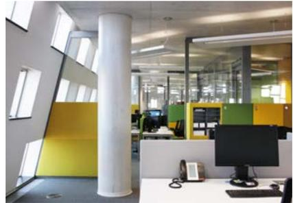
The building has a circular floorplan with an inward inclining façade. This facilitates the propagation of sound. To solve this issue, additional panels have been placed against the façade. (photo: Royal HaskoningDHV)
