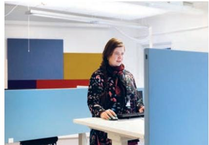
The use of acoustic panels will help to soundproof the office. Acoustic panels are made of sound-deadening materials that allow people to have a conversation in an open work area without immediately disturbing their co-workers. (photo: Anna Autio)
